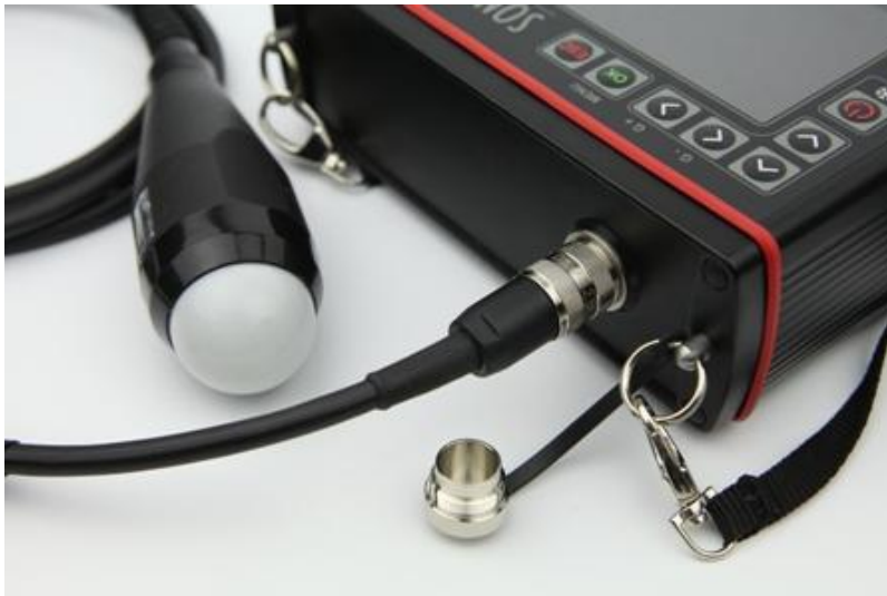
Probe correctly pinned up to the device
